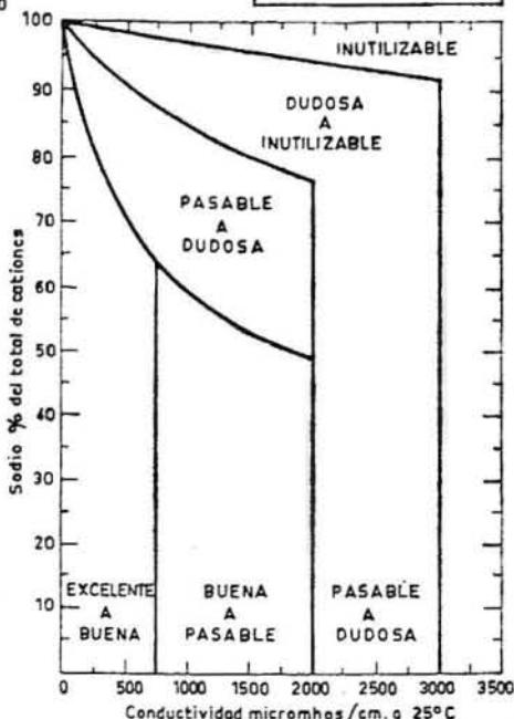
Adaptado de "THE QUALITY OF WATER FOR IRRIGATION USE" U.S.D.A.
